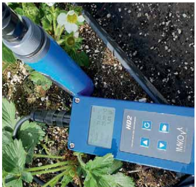
Cultivation of strawberries in an artificial environment and in the field / measurement of soil moisture with the HD2 by IMKO
