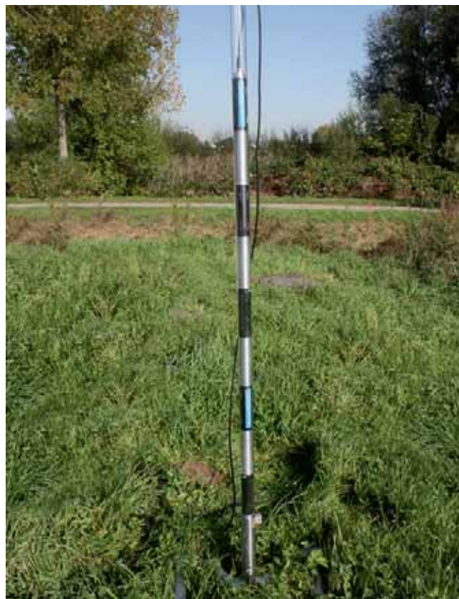
The PICO T3PN is the perfect compact and cost effective alternative for a lysimeter installation. The probe segments can be arranged to the prevailing examination pattern of the specific location, readings can be drawn by the particular depths.
