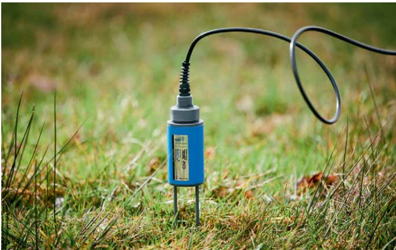
PICO64 for measurements in the topsoil - as a mobile probe, usually used with our HD2 handheld device or our Bluetooth® interface PICO-BT
