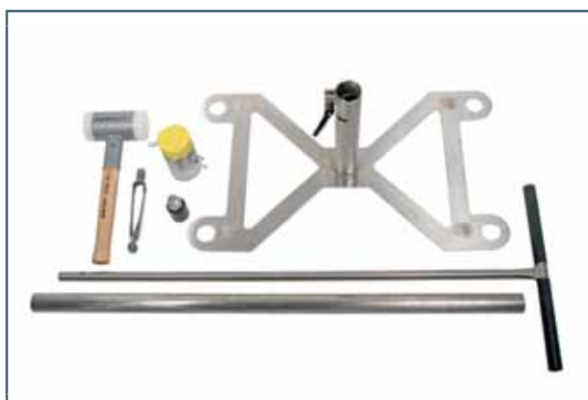
Auger equipment for precise and gap-free installation of the installation tube down to 1m depth
