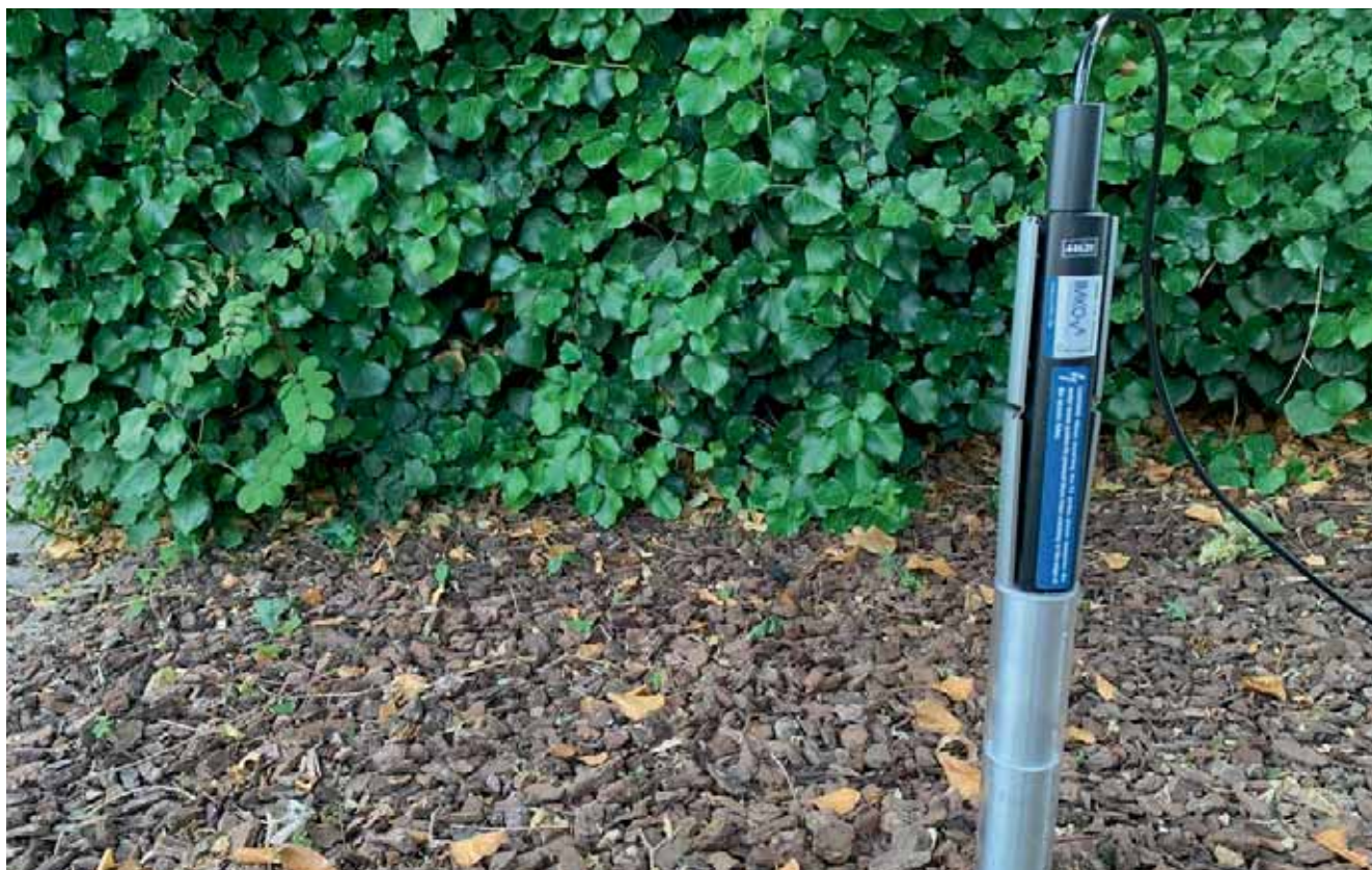
Installation of a PICO T3PN at the Reutgraben demo field – A comparative measurement of PICO32 / PICO64 at this location - visualization has been maintained through a microcomputer and local web application
