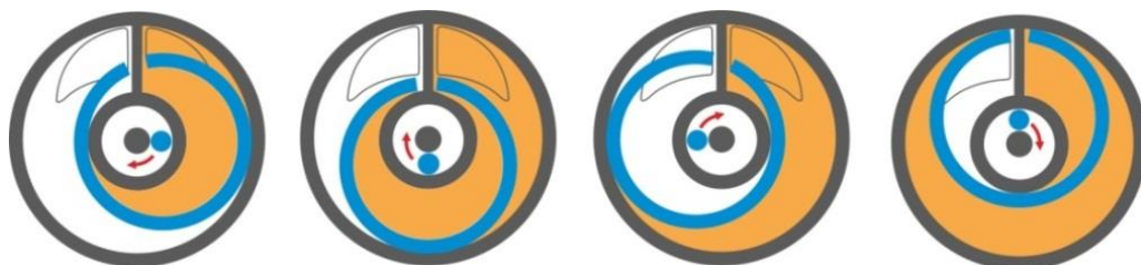
Figure 12 – DFM measuring chamber operation scheme
