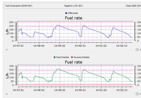
Example for a differential DFM D a) in Service S6 DFM software
