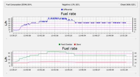
Example for a pair of single-chamber DFM CAN during differential measurement
