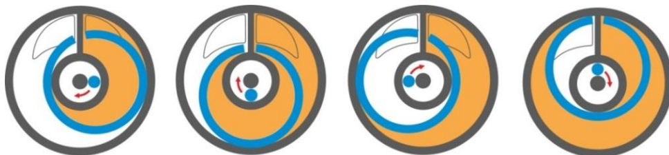
Figure 9 — DFM Marine measuring chamber operation scheme
