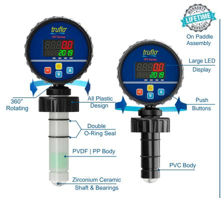
The TIM digital flow meters are easy to install with exceptional long life performance. Truflo TIM Series Paddle Wheel Flow Sensors are highly repeatable, rugged sensors that offer exceptional value with little or no maintenance. The TIM Series has a process-ready open collector signal with a wide dynamic flow range of 0.1 to 10 m/s (0.3 to 33 ft/s). The sensor measures liquid flow rates in full pipes and can be used in low pressure systems.
